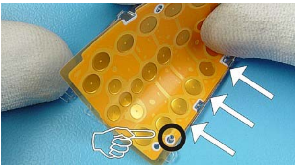
9. Place the DOME SHEET on the LIGHT GUIDE. First fit the hole in the DOME SHEET to the guide pin and place it congruent to the side of the LIGHT GUIDE ( see arrows ).
