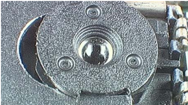
21. Remove the CAMERA MODULE with the SS-42 removal tool as shown in the picture.
