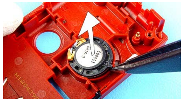
30. Remove the IHF SPEAKER with tweezers.
