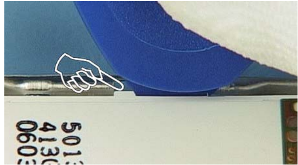
14. Use SRT-6 to separate the LCD-MODULE from the UI-SHIELD.
