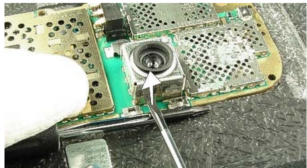
18. Use a slotted screwdriver as a lever to open the CAMERA SHIELD.
