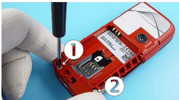
5. Unscrew the two Torx Plus® size 6 screws. For assembly, the reverse order and a Torx Plus® driver with a torque of 28Ncm has to be used.
