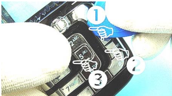
9. To remove the KEYMAT, use the SRT-6 to open the three snaps. Position 1. = two snaps, position 2. = one snap.
