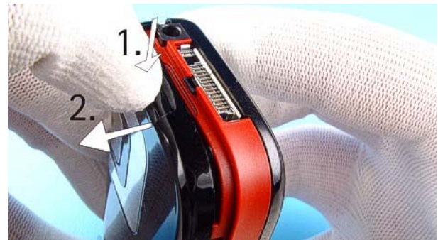
4. Press the C-COVER LOCK before pulling the C-COVER
