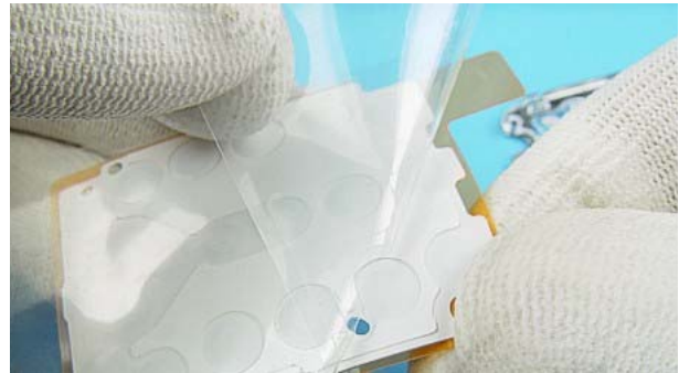
8. Carefully remove the transparent protection foil. Ensure that no residue remains on the transparent foil. Note! Do not touch the DOME SHEET after removing the foil.
